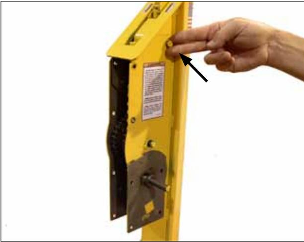
12. Reinstall right side outer plate 52-10 and lightly attach it to the frame using a single 1/4" x 1/2" bolt through the top hole -finger tight only.
