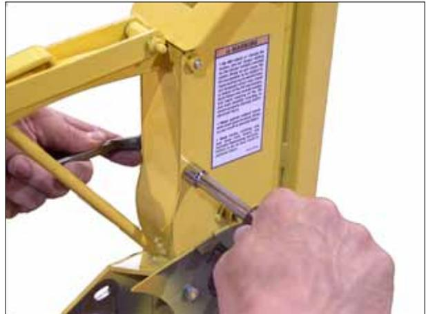
16. Tighten all of the 1/4" nuts and bolts as well as the 3/8" nut on the outer plates.
