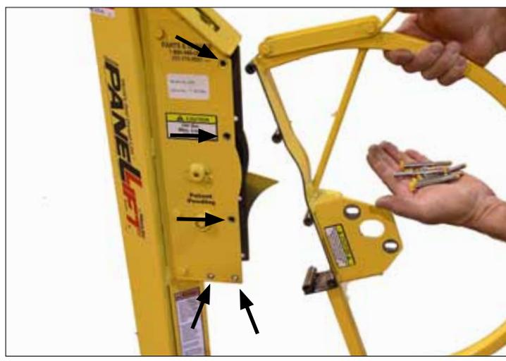
6. Remove nuts and bolts (five sets) and remove winch mount 52-13.
