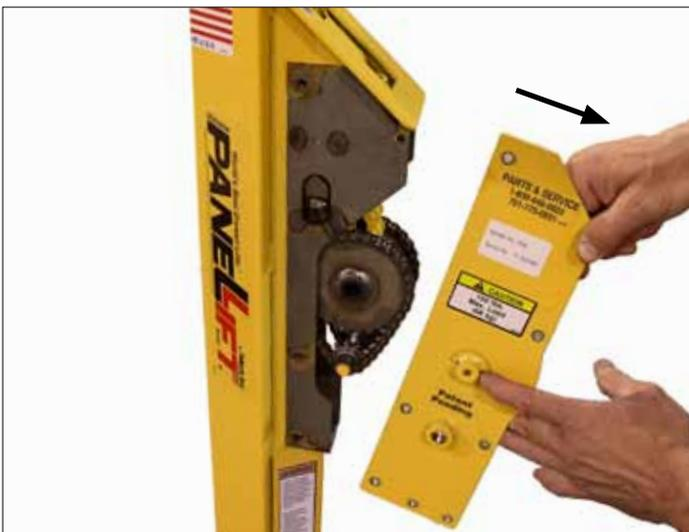
9. Remove left side outer plate with shoulder bolt. 52-10.
