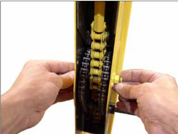
13. Jog and push the shoulder bolt through the assembly and tighten the 3/8" nut after the bolt has fully emerged from the right side outer plate. It is important that the bolt is carefully aligned with the bolt hole before you tighten this nut.
