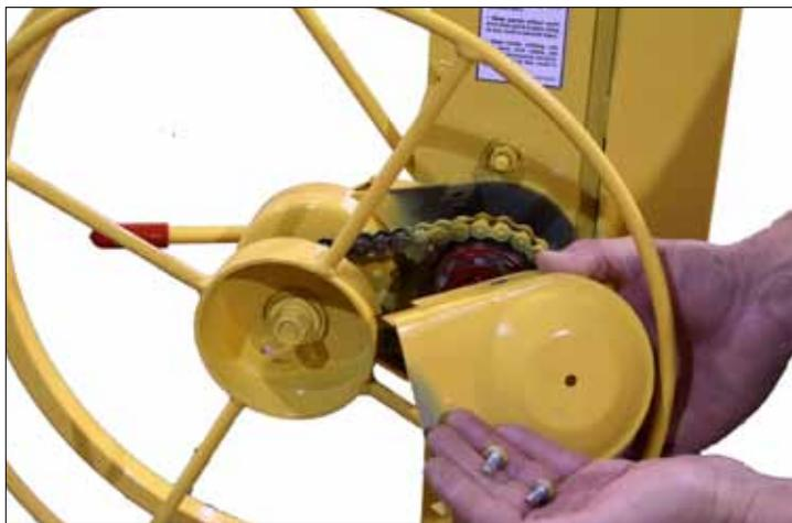
1. Remove the drive chain guard by loosening and removing top and bottom bolts.
