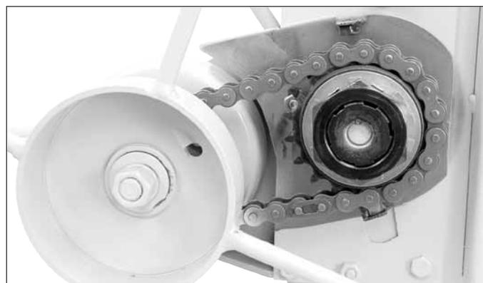
C. To check for proper tension, rotate the winch 1/2 turn to tension the lower portion of the chain. Move the upper portion of the chain up and down and measure the vertical movement of the upper portion of the chain midway between the sprockets. The correct distance of this movement should be approximately 3/8" to 1/2". If necessary repeat the previous steps until the correct tension is achieved. Replace the winch drive chain guard when the adjustment is complete.
