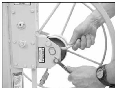
A. Lift the brake handle with right hand to allow the drive chain to find a neutral, tensionless position.
