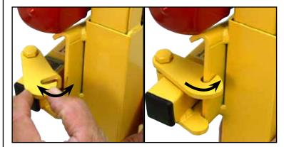
16. Secure the upper Cross Arm pocket of the Cradle behind the spring latch on the Upper Cradle Support.
