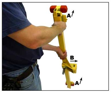
14. To load the Cradle, begin by holding it oriented as shown in the photo above with the tapered Cross Arm pockets ("A") away from you and the Pivot Box ("B") projecting to your right.
