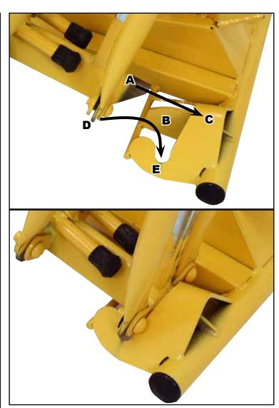
20. Store the Tripod Base Assembly as shown above. Angle "A" inserts beneath angle "C" while sliding over ridge "B". The Outer leg hinge points "D" will drop down into notch "E".
