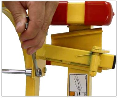
10. Securely tighten the bolt/lock nut assembly. Start with the lower bolts to minimize movement of the Upper Cradle Support Arm while tightening.
