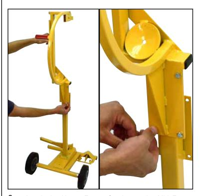
3. Attach the Upper Frame Section to the Mid Frame Section as shown using four 1/4" X 1/2" hex bolts and four 1/4" lock nuts.
