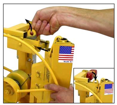
19. Lift up on the Frame Section Retaining Latch and tip the Frame Section into the locking position. Make sure the Retaining Latch is firmly holding the Frame Section in place.
