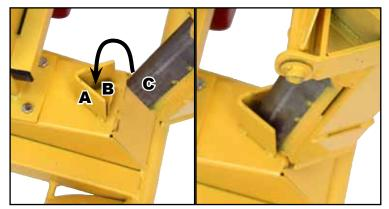
18. To load the Frame Assembly, start by mounting the foot of the Frame on the cart Base Section as shown. Angle "C" fits OVER angle "B" and inside angle "A".
