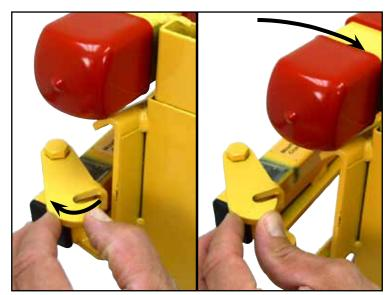
11. Check for a proper fit by opening the spring latch on the Upper Cradle Support and tilting the top of the Cradle away. The Cradle should move freely away without binding on the Upper Cradle Support and it should also remain securely in place when latched into the closed storage position. If adjustment is required, loosen the bolts and adjust as needed
