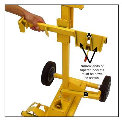
4. Attach the Cross Section to the Mid Frame Section as shown using four 1/4" X 1/2" hex bolts and four 1/4" lock nuts.
