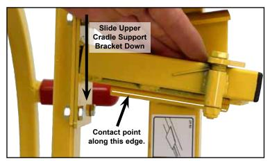
9. Slide the Upper Cradle support down on its slotted mounting holes until it makes contact with the edge of the tapered Cross Arm pocket on the Cradle. Due to variances in material, the contact point may be anywhere along the edge of the Cross Arm Pocket.
