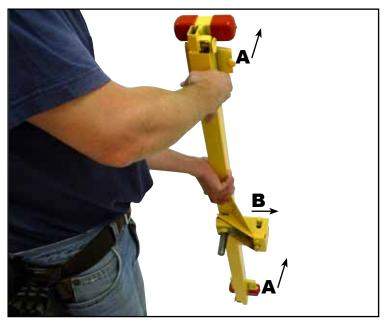
6. Begin by taking up the Cradle and holding it oriented as shown in the photo above with the tapered Cross Arm pockets ("A") away from you and the Pivot Box ("B") projecting to your right.
