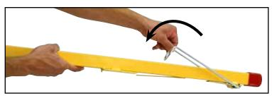
12. Begin with the Cross Arms. Fold the Support Hook backwards. This will prevent it from rubbing on the other components when the Cross Arm is stored.
