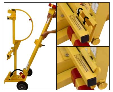
7. Mount the lower tapered Cross Arm pocket on the Lower Cradle Support as shown above. The narrow end of the Cross Arm pocket should face to the right toward the center of the storage cart.
