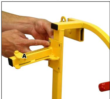
5. Attach the Upper Cradle Holder Assembly to the Upper Frame Section as shown using four 1/4" X 1/2" hex bolts and four 1/4" lock nuts.
