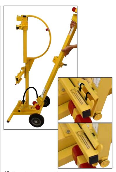
15. Mount the lower tapered Cross Arm pocket on the Lower Cradle Support as shown above. The narrow end of the Cross Arm pocket should face to the right toward the center of the storage cart.
