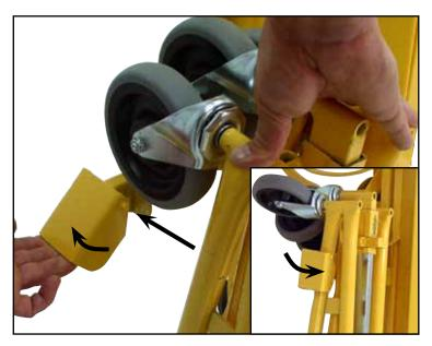
21. Lift the Tripod Retaining Latch and tip the Tripod base into the locking position.
