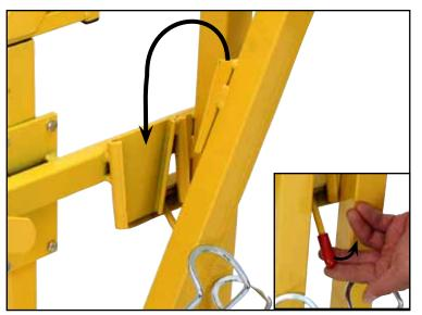
13. Insert the Cross Arm fully into the tapered pocket on the Cross Section until the spring tab on the Cross Arm locks into place. To remove, depress the Cross Arm spring tabs either directly or using the release arm provided.
